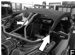
**Step 8:** Wrap Velcro mounts around the cage at the point they fall in: 1 in the front and 1 in the rear. Make sure the straps are securely fastened (Figure G).
