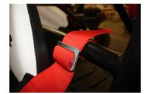
7) The next step is to get in and adjust your harness. While the car is off and set in park, put on the harness. (Note: in some cases you will need to loosen first). You will want to start by adjusting the Lap belts first. Lift up on synch buckle loop and pull slack down until belt lays flat across your lap. Repeat on both sides until belt is snug. (see photos below)
