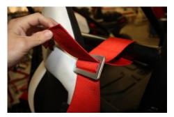
5) While keeping tension on first wrap feed slack through the bottom front side of buckle, pull tight. (see photos below)
