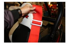
4) Wrap strap behind and over horizontal bar. Feed slack through the top of buckle from backside and pull tight. (see photos below)
