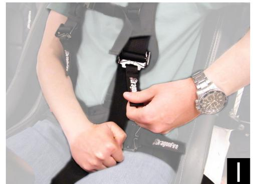
**Step 14:** Shoulder harness should be slightly below or even with shoulders to properly restrain occupant. (Figure J)
