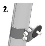
Put mirror mounting bolt through hole and place large rubber washer on the end of the bolt.
