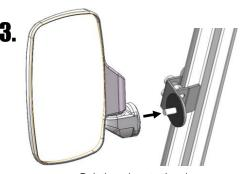
Bolt the mirror to the clamp but do not fully tighten yet.
