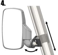
Slide mirror up or down Roll Cage tube to desired location. Rotate mirror on clamp to desired angle. When you are satisfied with the location and angle, tighten bolt.
