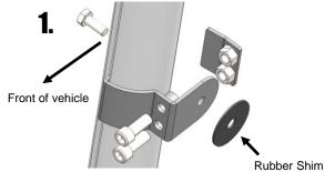
Disassemble clamp by removing the two 8mm socket head bolts. Place curved half of clamp against roll cage in desired mirror location. Insert bolts and thread into clamp plate with the welded nuts facing the bolt heads. Tighten bolts.
