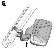
To tighten the folding feature of the mirror, tighten tension adjustment nut on the bottom of the mirror arm.
