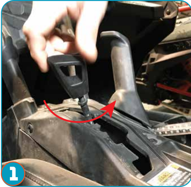
Remove OEM Shifter, turning the Shifter knob counter clockwise until it clears the screw.
