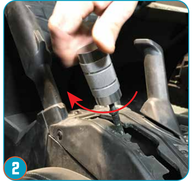
Screw on New X3 Shifter (clockwise) until knob is tightly secure.
