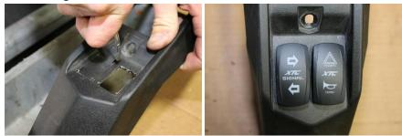
10. **Install Switch Harness** – Plug the large switch connector into the Control Module and run the Switch Connectors to the switches. Apply grease to the Switch Terminals and plug switches into connectors and re-install plastic cover.
