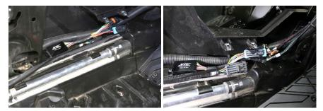
8. **Run power wire** – Plug the two pin Power Connector into the Control Module, run the other end up to the OEM busbar under the dash. Attach the ring terminal with the Red Wire to the left Keyed Power Post and the Ground to the Right Ground Post, do not connect to the center full time Power Post.
