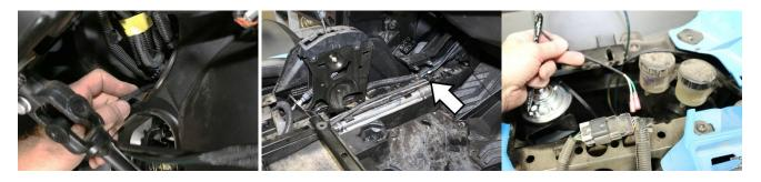
7. **Mount the Control Module**— Using the provided screw or cable tie mount the Control Module next to the main wire harness, Plug the front and rear harness in.
