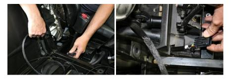
3. Run the other ends – of the rear harness with the Yellow wire to the driver's side panel, the one with the Green wire is run to the passenger side panel under the plastic rear panels that were removed where the cage goes into the plastics. Un-plug the factory harness and plug our harness in-line on both sides.
