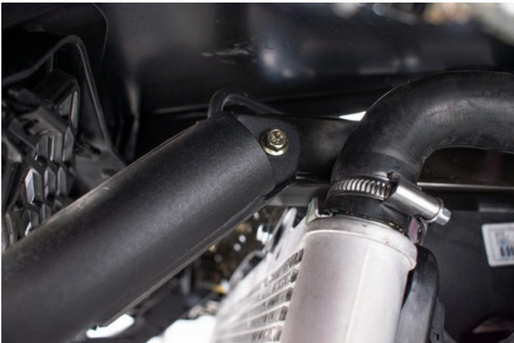
4. Remove the mid mounting points along with the spacers.
