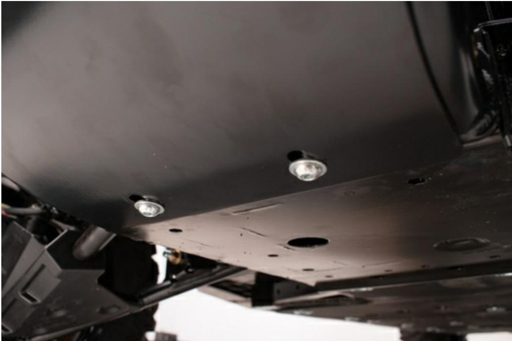
**Note:** If installing a winch and fairlead at this time use the hardware provided with the fairlead to secure the upper mounting points for the skid plate.
