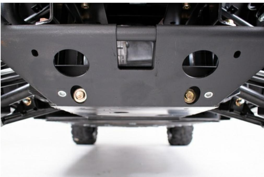
6. Lift and pull forward on the inner bumper to remove it from the vehicle. There are 2 wire hooks built into the bumper holding it onto the frame of the vehicle.
