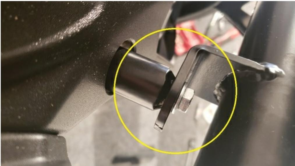
4. Secure the rear mounting tabs of the left and right support bars to the unused holes in the vehicle's frame just above the rear upper control arms using (1) M8x20 Hex Bolt, (1) 5/16" Fender Washer, (1) 1/4" Washer, and (1) M8 Nyloc Nut for each side. The 5/16" Fender Washer will go against the head of the bolt then pass the bolt through the rear of the frame and support arm followed by the 1/4" Washer and Nyloc Nut.
