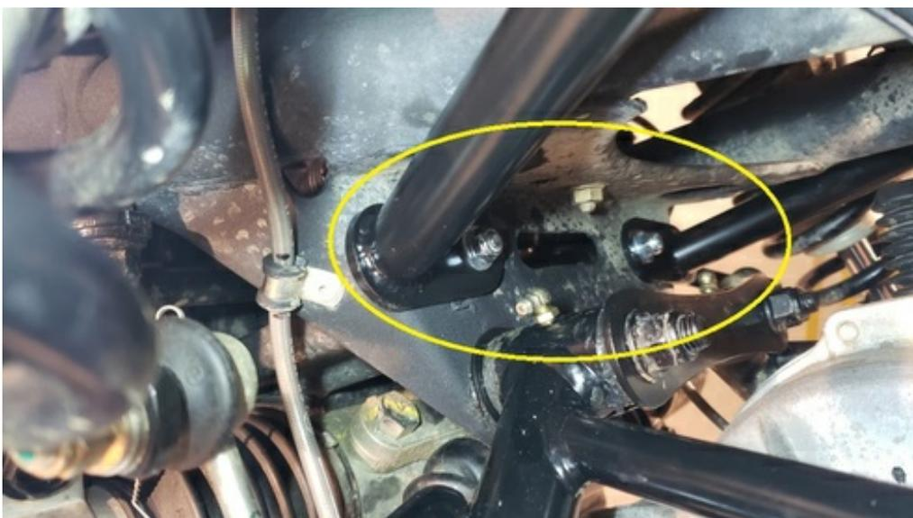
5. Check the alignment of the support bars relative to holes drilled in the front fascia, adjust the rotation as necessary then tighten the hardware at the rear mounting tabs installed in the previous step.
