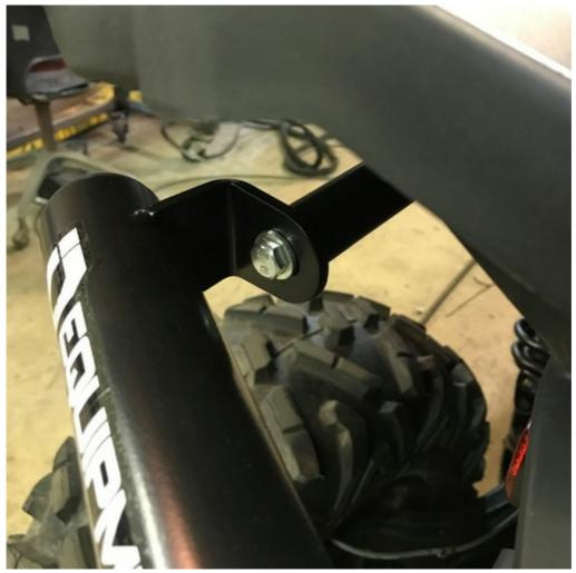
5. Tighten the original radius rod/rear plate nuts.
