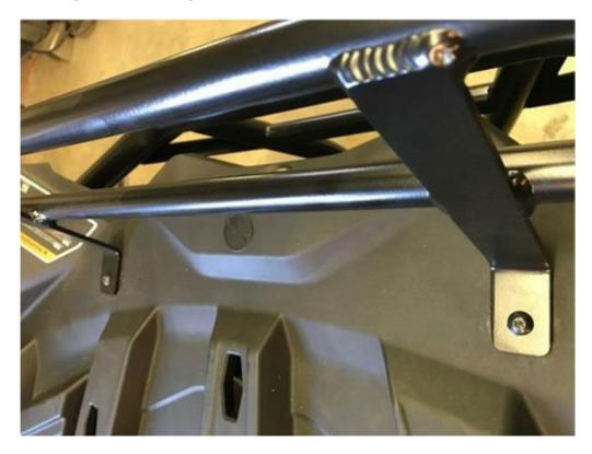
4. Line up the previously installed clamps with the cargo rack and install the supplied allen head bolts.
