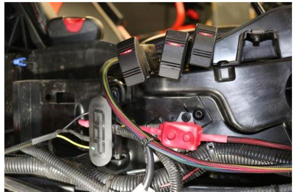
9. Run the power wire from the fuse block to the factory busbar fulltime power( Center Stud), secure the 50 amp Circuit Breaker with the supplied screws.
