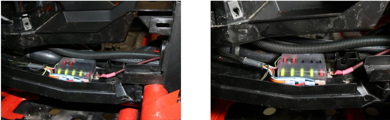
5. Mount the barrier strip on the dash support 1.25" bar with the provided self tapping screws.
