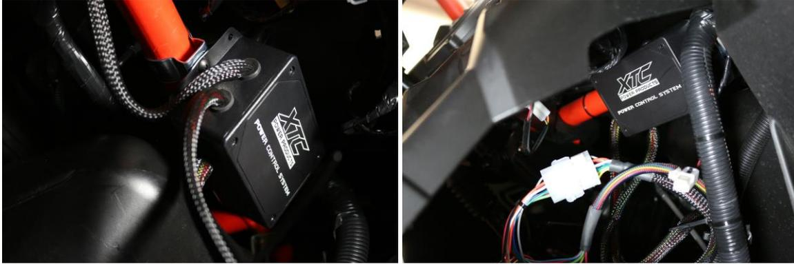
Tighten both clamps and tighten the two 10-24 mounting screws
