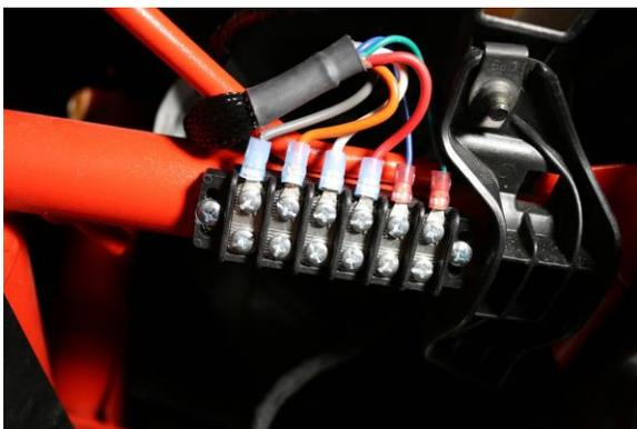
6. Connect the power wire from the devices to be controlled to the appropriate terminal on the barrier strip. Switch 1 through 4 should be used for your larger accessories and are on power relays, switch 5 and 6 the power goes through the switch and should be used for smaller items like whip light, interior lighting or stereo. The following is the switch designations.
