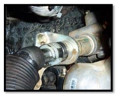
e. Pull boot back over the ball joint and steering stop and refasten with 11" zip tie. Be sure to verify the zip tie is tight so prevent material from getting into the boot.
