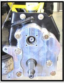
d. Loosely fasten the all four bolts with ½" flat washers and ½" lock nuts. Recheck all parts that were used and make sure everything fits correctly, and then go ahead and fasten all bolts. (3/4)[105 ft lbs]
