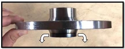
c. With the shorter lip side faced down, find the bolt pattern that corresponds to your make and model with the provided studs PGLC-WSTUD-103 (10mm-1.25 stud) (4/137mm bolt pattern)
