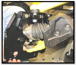
g. Now you can fasten the upper ball joint mounting bracket. (5/8)[70 ft lbs]
