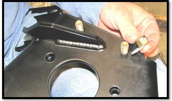
e. Properly position the lower ball joint into the lower ball joint mounting bracket on the backing plate assembly. Insert the axle into the backing plate. Then fasten the front lower ball joint with the factory hardware. (15mm)[50 ft lbs]
