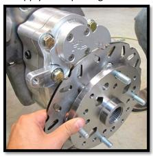
a. Slide on the supplied **30mm lock washer**, followed by the **30mm spindle castle nut**. (46mm) [**Min 120 ft lbs**] Tighten the castle nut further if needed to align grooves with holes in the spindle for the cotter pin. Install the supplied **cotter pin**. Both ends of the cotter pin must be folded.
