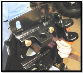
e. Retighten the upper ball joint mount bracket to the backing plate. Check the camber again. If it's correct, proceed to step #11. If not, repeat the previous step until you achieve the correct angle.
