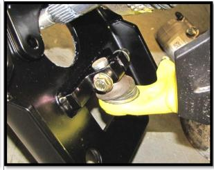
f. Place the upper ball joint into the upper ball joint mount bracket. Fasten it with the factory hardware. (18mm)[90 ft lbs]
