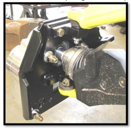
e. Install the tie rod end into the backing plate tie rod mount bracket. Fasten the tie rod end with the factory hardware. (18mm)[90 ft lbs]
