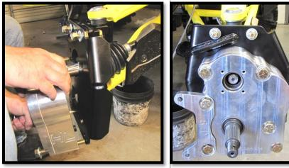
d. Loosely fasten the all four bolts with ½" flat washers and ½" lock nuts. Recheck all parts that were used and make sure everything fits correctly, and then go ahead and tighten and torque all bolts. (3/4)[105 ft lbs]
