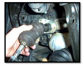
d. Place the steering stop clips (2ea) between the inner tie rod joint and the rack and pinion. It is a tight fit, so you may have to force it on this is to ensure that the spacer stays in place.
