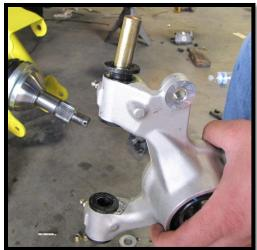
Now insert the bushings and pivot tubes into the new collar mount bracket and backing plate.
