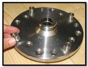
f. Locate a **brake rotor PGLC-ROTOR-2**. The side with the counter bores should be facing up. Place the rotor on to the hub and line the holes up with the tapped holes.
