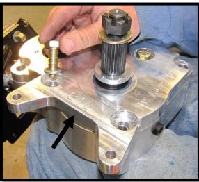
d. Insert the washers and bolts below through the remaining four holes in the front of portal box.
